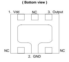
Note: 3. NC is "No Connection" which is recommended to be tied to ground.
